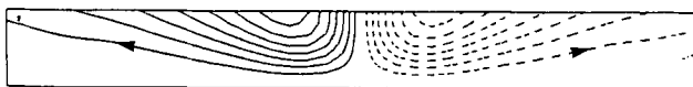
FIGURE 18. Streamlines in the (x_2, x_3) -plane of the first eigenfunction. x_2^+ = 65 corresponds to the top of the figure (from Moin 1984).
