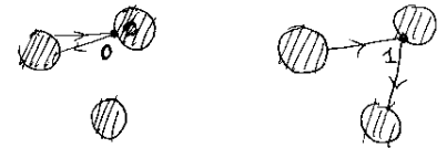
Figure 1.4: Binary labeling of the 3-disk pinball trajectories; a bounce in which the trajectory returns to the preceding disk is labeled 0, and a bounce which results in continuation to the third disk is labeled 1.
