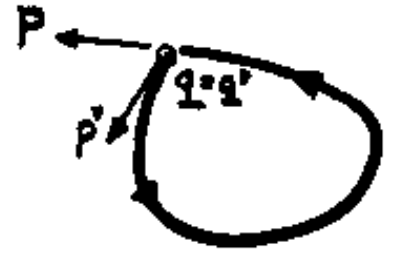
Figure 26.1: A returning trajectory in the configuration space. The orbit is periodic in the full phase space only if the initial and the final momenta of a returning trajectory coincide as well.
